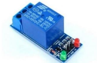
**Gambar 4.** *Relay Module*
